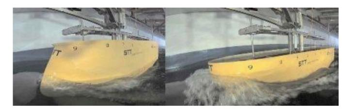
The X-Bow "pierces" the surf and disperses its energy to the sides of the boat. That means there's less of a rocking motion, which in turn reduces motion sickness.
